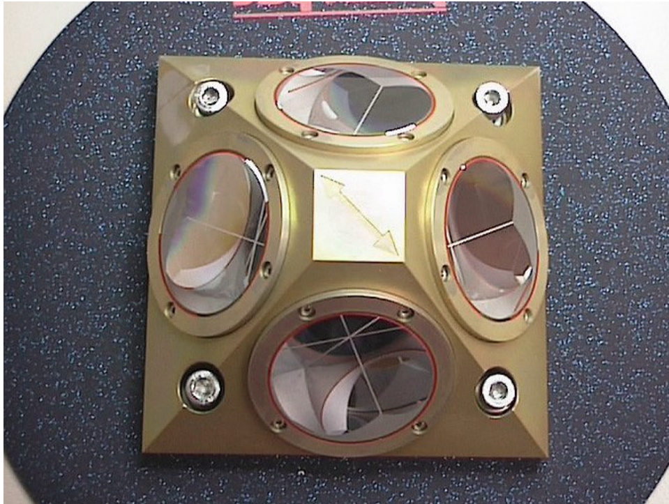
Figure 1 The CHAMP Laser Retroreflector Array
